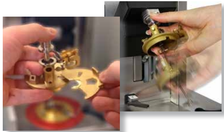
Easy disconnection, for easy and external cleaning of the cup-cover
