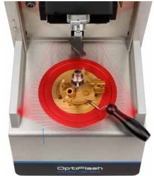
Optical fire detecting system covers entire hot area
